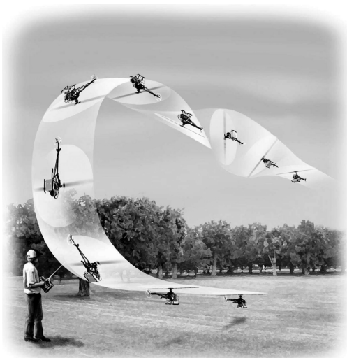
Fig. 1 Split-S maneuver, which consists of a half-roll followed by a half-loop; result is a reversal of the flight direction (picture courtesy of Popular Mechanics Magazine ).
